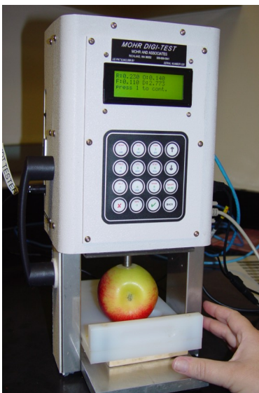
MDT-1 measures the crispness and firmness of apples. Photo: Kate Evans, Wash. State Univ.
