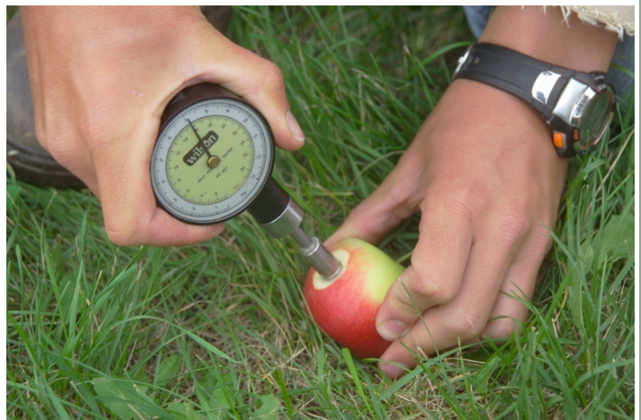
Penetrometer measures firmness of apple flesh (Photo credit: David Hansen, University of Minnesota)
