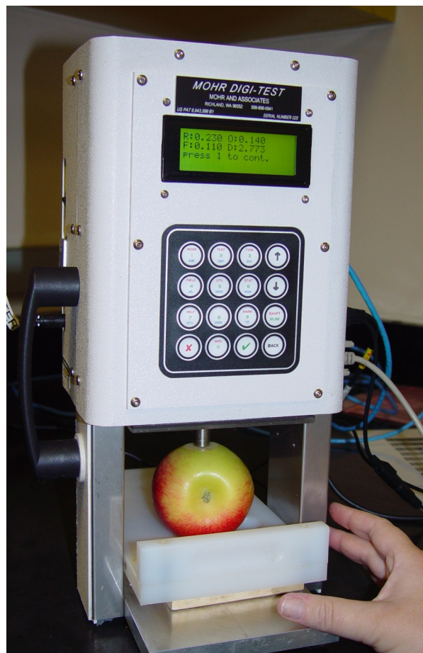
Figure 2. Evaluating crispness with a Mohr Digi-Test.
